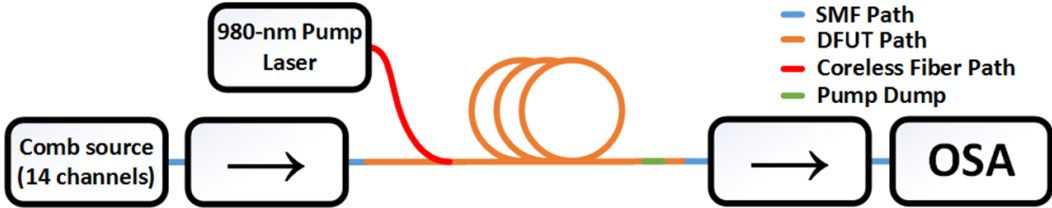
FIGURE 1.8 – Setup used to measure the gain and NF of fiber A and B.
