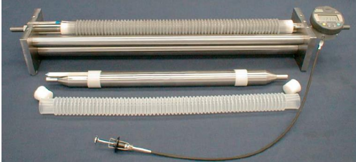
Figure 1-21. A corrugated PE-mold and a 425 mm reference bar according to the ASTM C1698.
