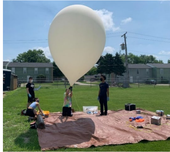
Figure 9 The research team preparing a flight by filling up the balloon. As seen in the figure, one person must hold the balloon at the base during the filling period to stabilize the balloon. Note gloves are worn during the filling process as to not place any oil onto the latex of the balloon.
