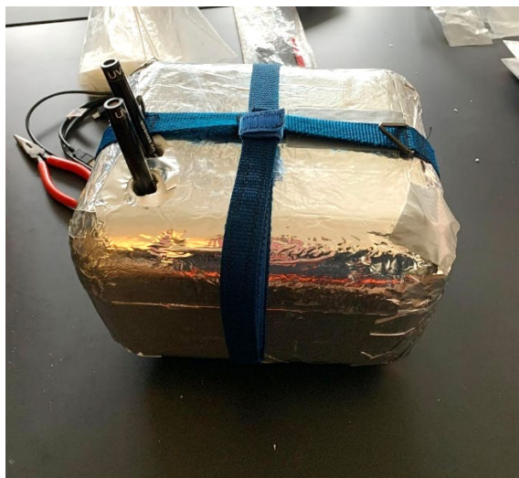
Figure 2 Example of payload used in launch. This payload has a harness on it to keep it closed during the flight. Atop the payload two UV radiation sensors are placed to collect UV radiation data throughout the flight.
