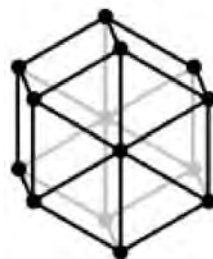
Figure 1: Hexagonal symmetry commonly found in zinc oxide structure
