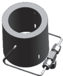
Figure 2-8 In-house modified sputter head.
