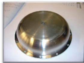
Figure 2-9 Exchangable apertures as developed in-house.
