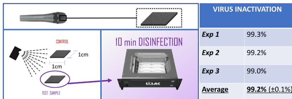
Figure 3. Representation of the spray deposition of virus onto a foam from the inside of the microphone, and representative results from disinfection experiments.
