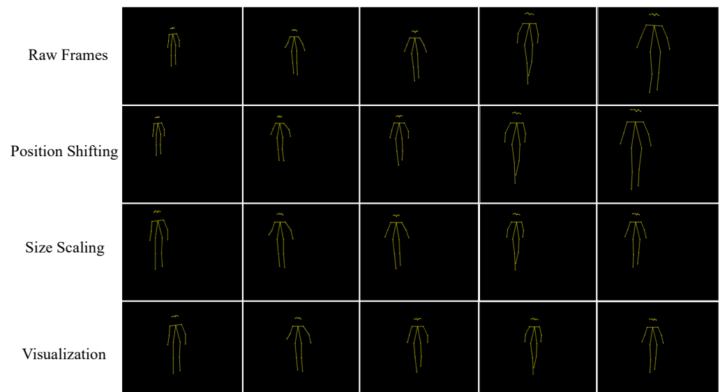
Figure 2. Example of several frames of an EOA patient walking towards the camera illustrating the effect of the different normalization steps when using the ASH method.
