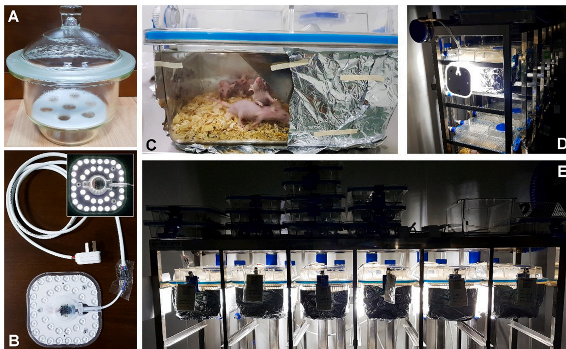
Fig. 1. Experimental setup for skin phototoxicity analysis in nude mice. (A) Anesthesia induction chamber. (B) LED panel (18 W) that was used as a source of light to emulate typical outdoor and indoor lighting conditions that photosensitized patients could be exposed to, producing an incident illuminance of 3982–5033 lx (mean \pm SD = 4558 \pm 537 lx) at the level of the animals. The insert shows the LED panel in on mode. (C) Cage setup with the created window to which the LED panel was affixed for light exposure. The sides and bottom of the cage were covered in aluminum foil. (D and E) Individual ventilated cage setup during the skin phototoxicity study, which lasted 24 h. Active climatization of the cages prevented animal exposure to hyperthermic conditions.
