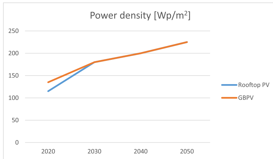
Fig. 8. Future development of rooftop and ground-based PV power density till 2050.
