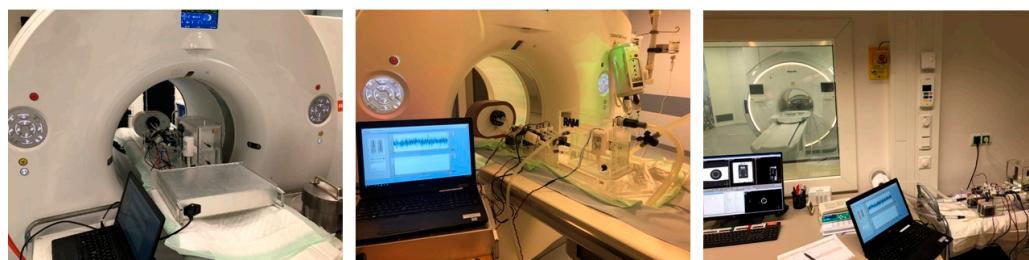
Figure 3. Example of the overall phantom measurement setup in PET/CT (left), CT (middle) and MRI (right).
