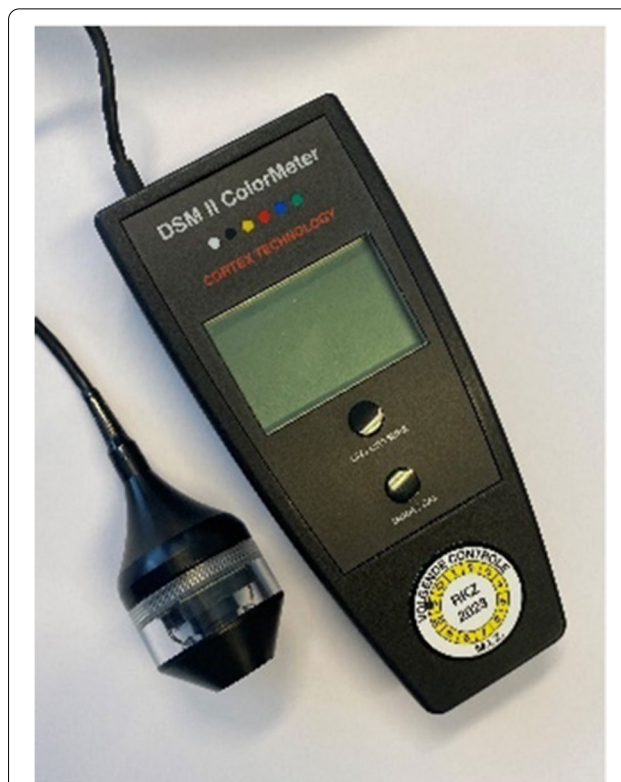
Fig. 7 The DSM II Colormeter measures scar color and pigmentation by calculating an erythema and melanin index (Cortex Technology, Hadsund, Denmark)
