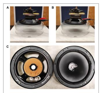
**FIGURE 1** | Environmental Treatments—No Noise and Noise Signaling Environments. The mating arenas were set on a granite platform with the speakers held on top of the arena with mechanical arms (**A**,**B**). One of the speakers had the speaker cone removed (**A**,**C** left) and thus did not introduce air particle movement. The other speaker had the speaker cone intact (**B**,**C** right) and introduced air particle movement. All trials were run in the dark.
