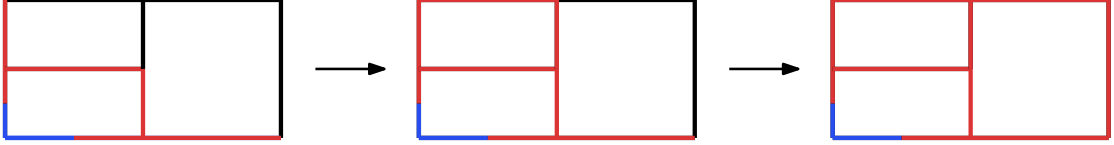
Figure 9.3: Output computation of a box when inputs are empty. First we can compute the outputs of the top left box and then the outputs of the right box. In this example, we then know that the curves have a Fréchet distance greater than \delta as (n, m) is not reachable.
