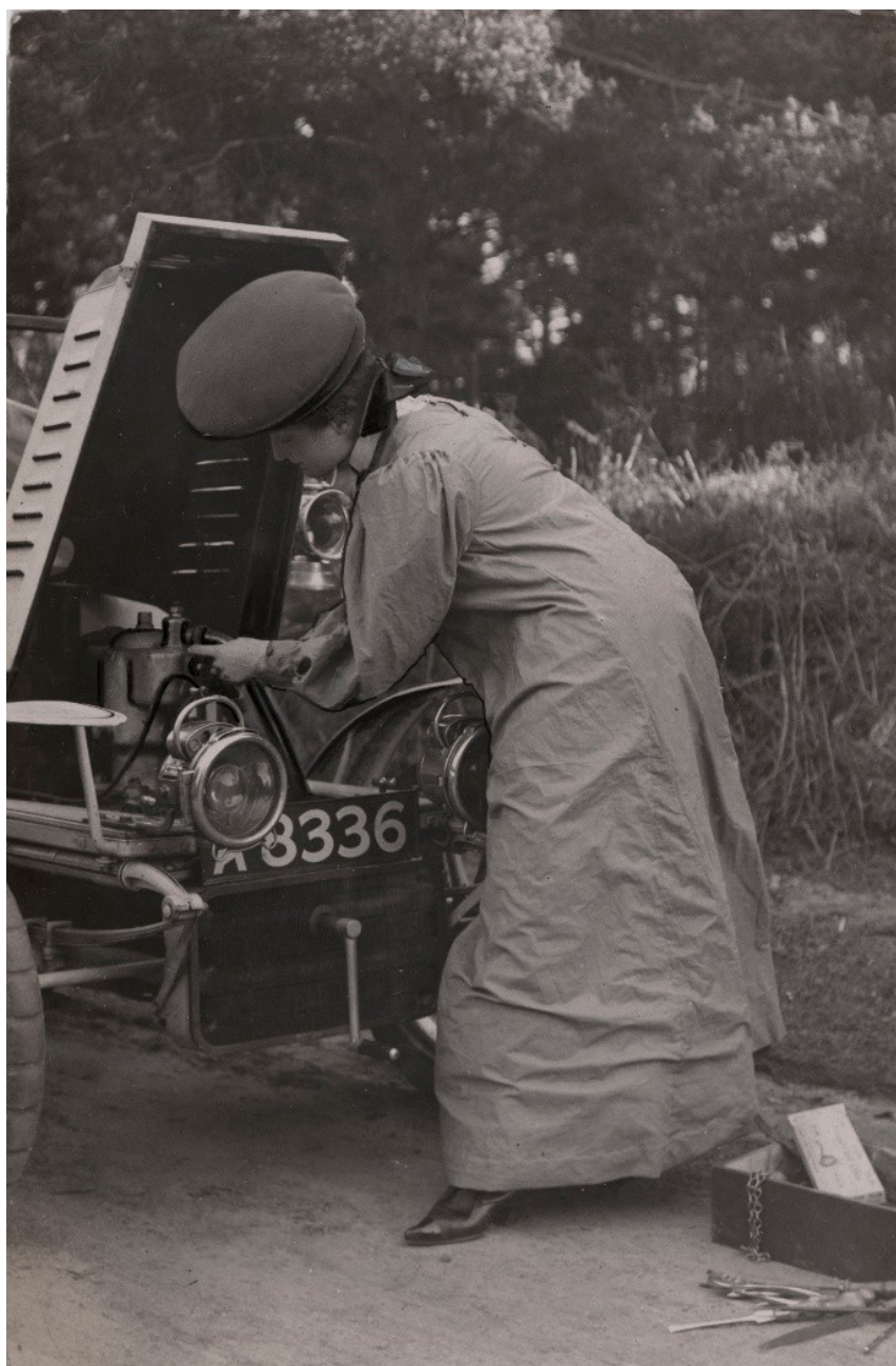
Figure 4.28. 'It is a simple matter to remove a faulty sparking plug', Nicholls family archive, Folio No. 276.
