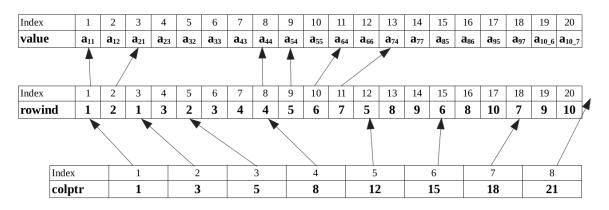
Figure 3.7: CSC data structure of intersection matrix shown in Figure 3.3
