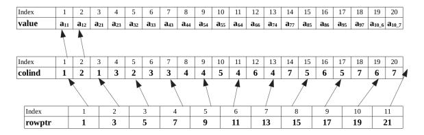
Figure 3.6: CSR data structure of intersection matrix shown in Figure 3.3
