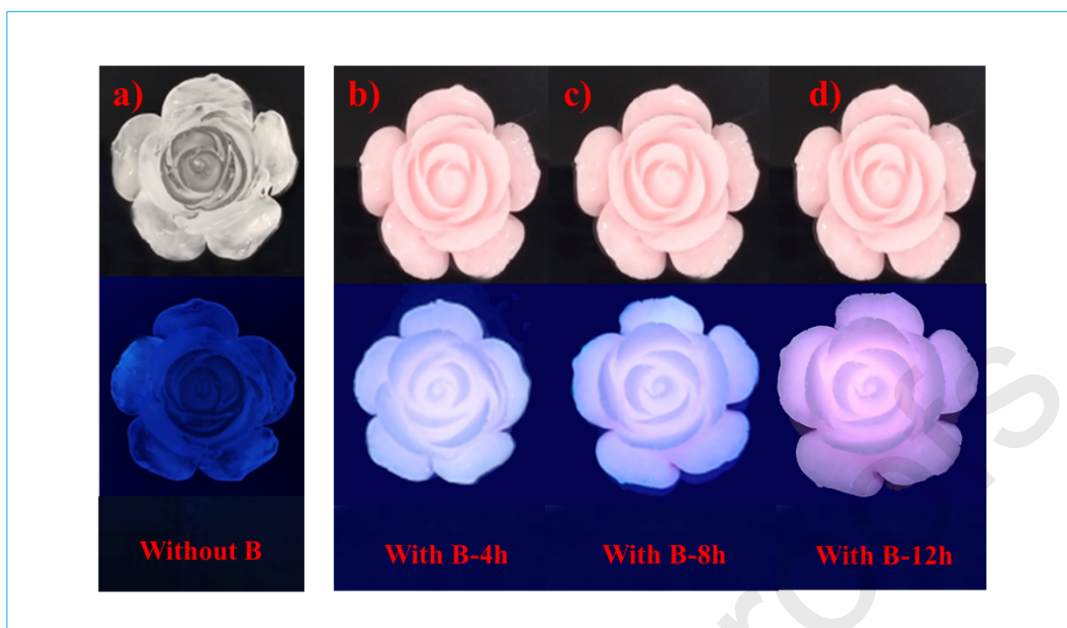
Figure 9. 3D printed roses without (left) and with (right) PDI-C6@Q[8]@QSD, where a indicates roses without PDI-C6@Q[8]@QSD, photographed under daylight (top) and 365 nm (bottom) UV-LED light, and b, c, and d indicate roses with PDI-C6@Q[8]@QSD at 4, 8, and 12 h, photographed under daylight (top) and 365 nm (bottom) UV-LED light.
