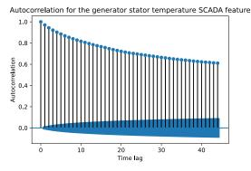
Figure 2: Auto-correlation for the generator stator temperature time-series. The components are significantly non-zero, signifying non-random nature of the metric.
