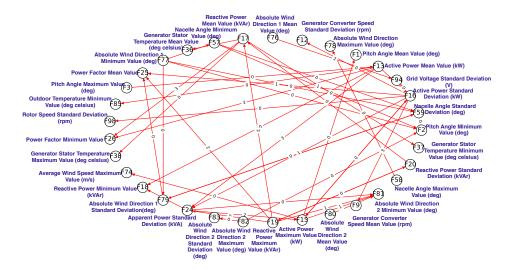
Figure 4: Identified temporal causal relationships in SCADA data during Yaw System anomaly using the proposed learning model. Here, the relation  $p \rightarrow q$  would signify that p is causally affected by q.
