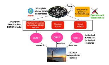
Figure 3: Proposed technique for identification of hidden causal confounders in SCADA data.
