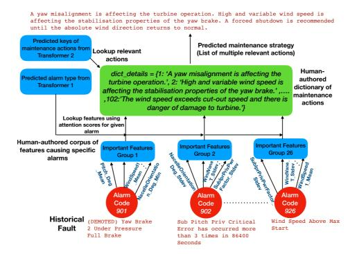
Fig. 5. Development of templates for maintenance actions
