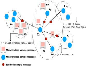
Fig. 4. Illustration of synthetic minority oversampling for wind turbine alarm messages
