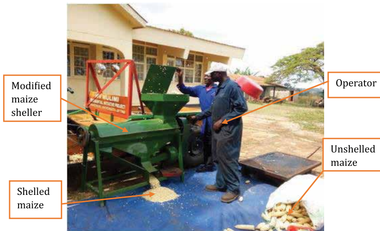
Figure 6. Operational view of the modified multi-purpose vehicle maize sheller [1].
