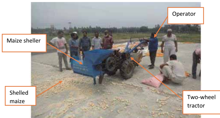
Figure 8. Operational view of the two-wheel tractor mobile maize sheller [9].
