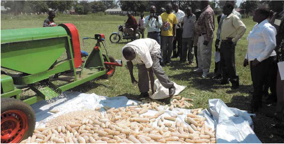
Figure 9. Operational view of the Munyegera Agro-Machinery mobile maize sheller [10].
