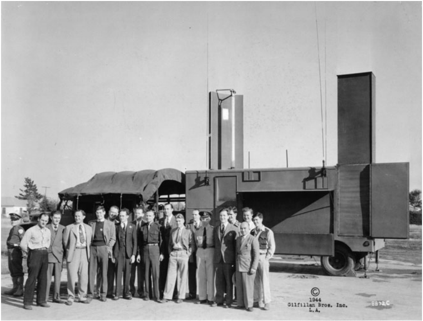
Figure 6.2. AN/MPN-1 #1, at the Gilfillan plant in Los Angeles. The trailer contained the search radar (upper left), the precision azimuth antenna (lower center), and the precision elevation antenna (upper right), in addition to the operators' position (internal). The truck contained the power generators and air conditioning units. The individuals are not identified. Author's collection.
