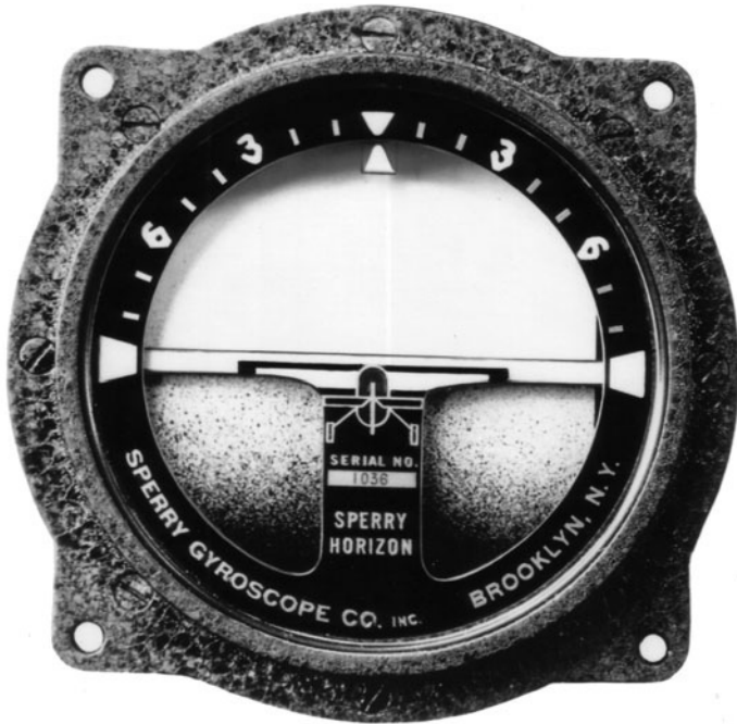
Figure 1.2. Sperry artificial horizon. Reprinted with the permission of Unisys Corporation, courtesy National Air and Space Museum, Smithsonian Institution (SI 99-41447).
