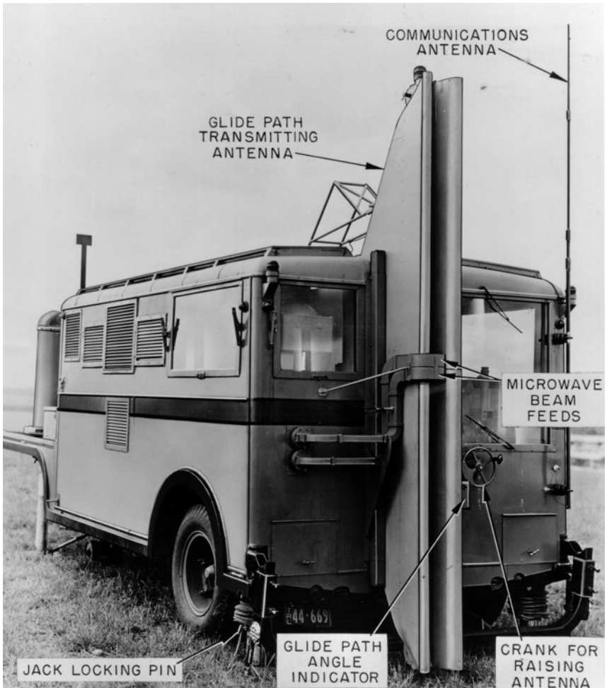
Figure 5.4. The Sperry Gyroscope microwave glide path transmitter. Note that the original horn radiators have been replaced by what is essentially a vertical “slice” through them. With microwave transmission, the width of the beam is inversely related to the transmitting antenna’s dimensions. In this case, the antenna produced a pattern that was wide horizontally but very narrow vertically. Courtesy of Hagley Museum and Library.
