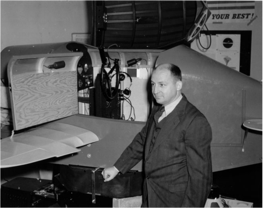
Figure 1.4. Ed Link posing with his “blue box,” an early blind flight trainer. National Air and Space Museum, Smithsonian Institution (SI 99-4151).
