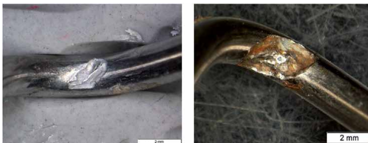
Figure 8. Typical tribocorrosion in the friction area of a stainless steel net after some months in the Pacific Ocean [12].
