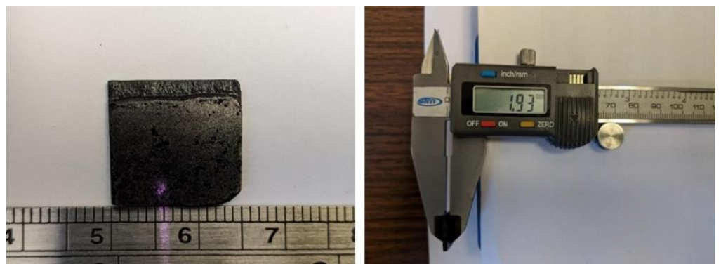
Figure 7. Appearance and dimensions of a cut and smoothed 3D printed magnetic composite with three print layers.
