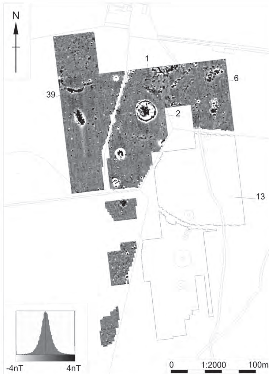
Figure 3.2 Gradiometer survey of Knowes of Trotty. Anomalies 1 and 2 represent Mound 1, the largest of the barrows, and anomaly 6 the early Neolithic house.
