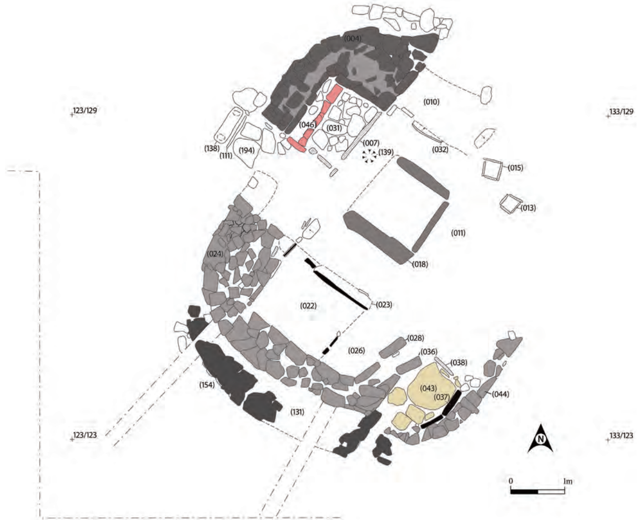
Figure 7.18 Plan of modified Red House, showing different constructional elements (red shows area of red-clay rendering).
