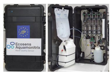
**Figure 7.** Outer and inner view of an integrated IoT sensor for water quality monitoring applications. The sensor consists of a nitrite and nitrate analyzer based on a novel ion chromatography method, used for detection of toxic substances [112].
