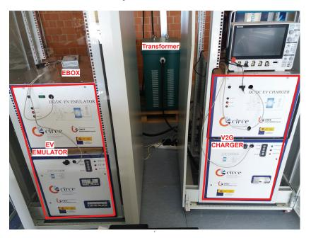
**Figure 12.** General overview of the testbench used for the power tests done with the proposed EVE. On the left, a 50 kW EVE together the EBox gateway; On the right the HUT system built up with a 50 kW V2G charger; and the power transformer in the centre.
