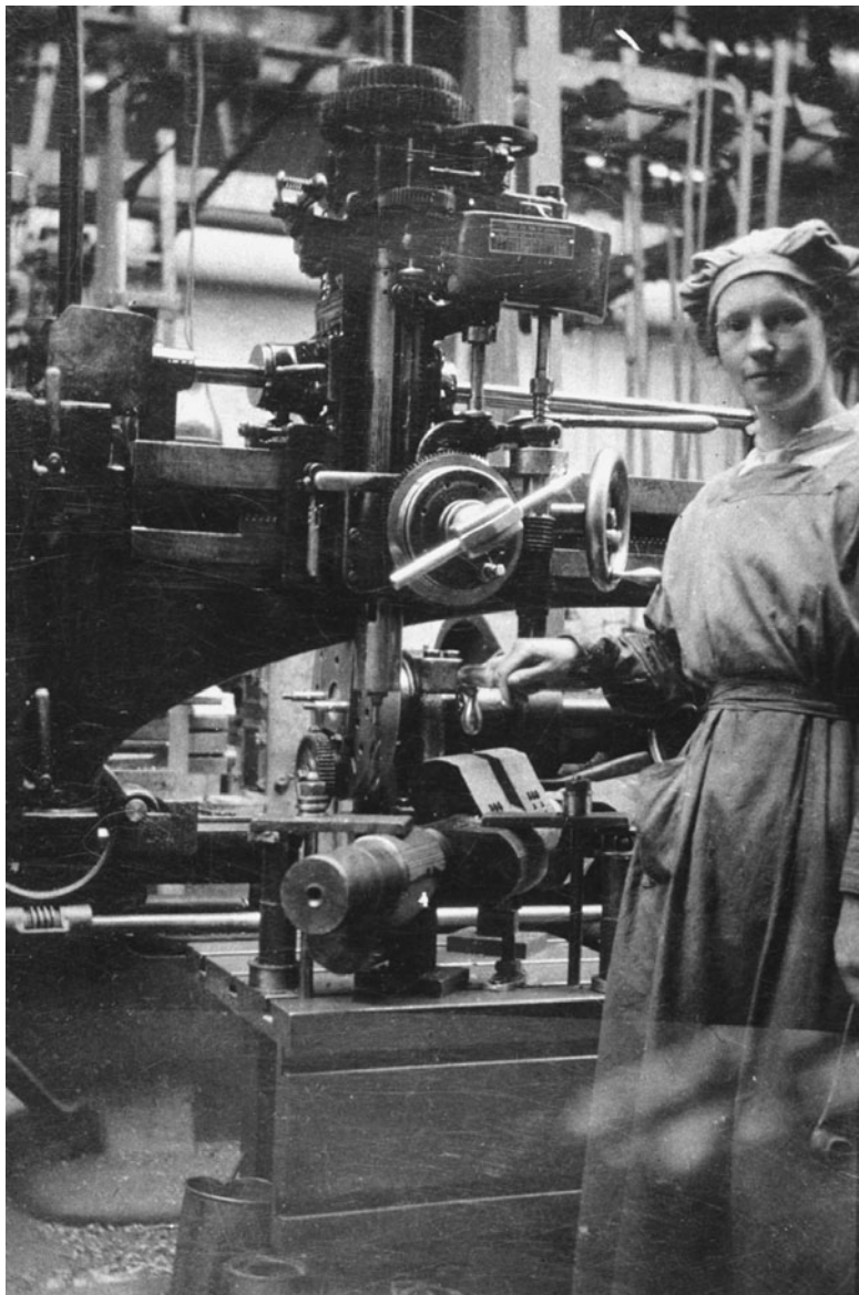
“A paradise for the woman engineer.” Boring engine connecting rod forgings at the Tongland Factory, Scotland. Engineering , 9 November 1917. By permission of the National Library of Australia.
