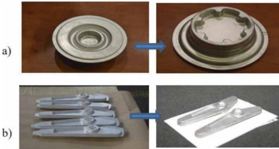
**Figure 16.** View of forgings from AZ31 alloy: a) semi-hub of wheel, b) lever after process at beginning temperature of 410°C [28].
