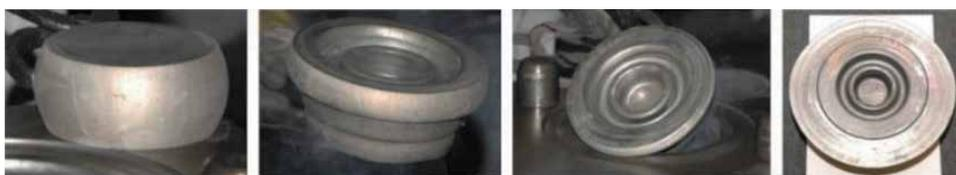
**Figure 17.** Stages of forging of AZ31 semihub of wheel, for aeroplane at temperature of 410°C.
