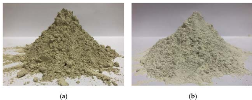
Figure 2. Typical photos of (a) fly ash powder, and (b) calcined lime mud powder.
