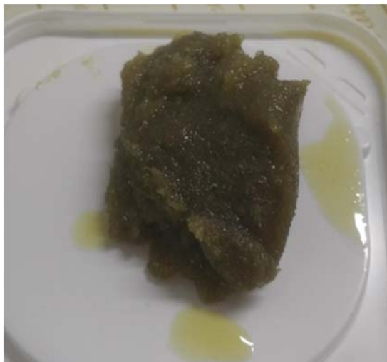
Figure 5. Fine sample of polyurethane foam soaked with 20w50 oil after oil sorption long test.
