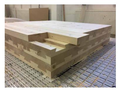
Figure 4. Adhesive- and metal fastener-free dovetail wood board element.
