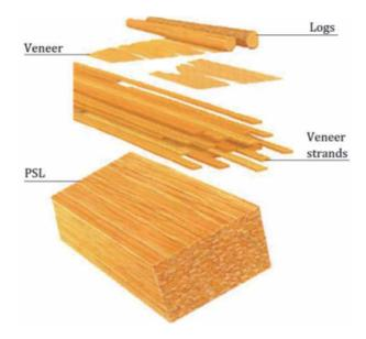
Figure 11. Orientation of veneer strands in PSL (source: photos obtained from WorldPress.com [50]).
