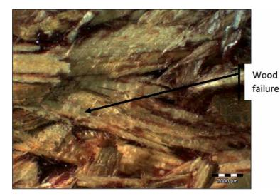
**Figure 8.** *Failure occurred in the wood portion.*  Size Effect of Core Strands on the Major Physical and Mechanical Properties of Oriented Strand... DOI: http://dx.doi.org/10.5772/intechopen.99953
