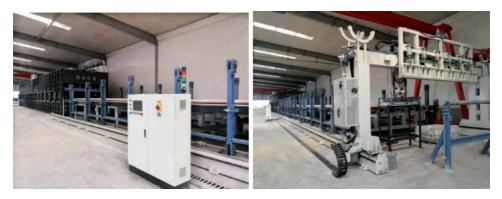
Figure 5. CLT press (source: Photo obtained from Yantai Bohai woodworking machinery Co., ltd).
