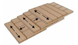
Figure 6. Generic CLT configuration.
