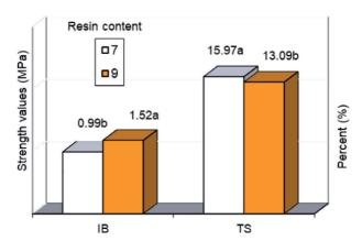
Figure 11. Effects of resin content on internal bond and thickness swelling.
