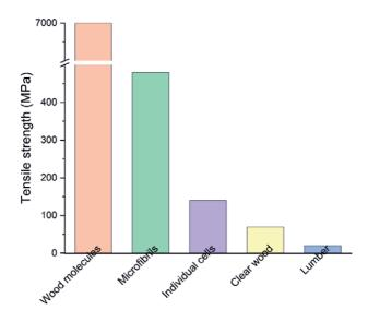
**Figure 9.** *Tensile strength of wood at various levels.*
