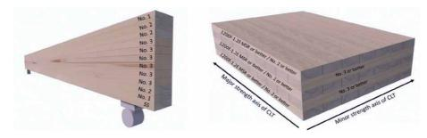
Figure 11. Design of GLT (left) and CLT (right) [9].
