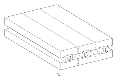
Figure 9. Dovetail wood elements as floor slab alternatives-4 (hollow type-2).
