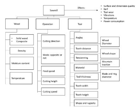
**Figure 4.** *Factors in a sawmill monitoring.*
