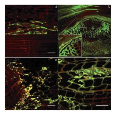
**Figure 27.** Images of particleboard section glued using fluorescence-labelled UF resin, bar = 50  $\mu$ m [63].
