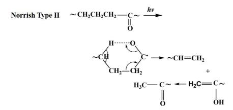
Figure 10. The reaction mechanism for photochemical degradation of polymer in WPC [24]. crystallization of smaller polymeric units and individual monomers, reducing the mechanical properties of the WPCs [24]. Some chemical additives, such as photostabilizers, antioxidants, and pigments have been incorporated into WPC matrices to retard the discoloration of the composites.
