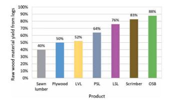
Figure 2. Raw wood material yields of sawn lumber and EWPs from logs (data from [7, 8]).
