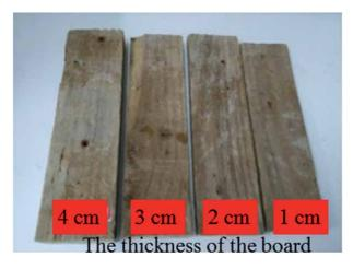
Figure 6. The timber board of ancient building with different thicknesses.
