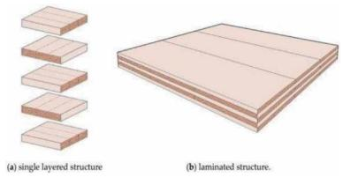
Figure 2. Cross-laminated timber [46].
