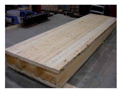
Figure 9. CLT panel layup with box-based configuration (adapted from Chen [11]).
