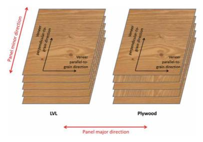
Figure 8. Layups of LVL and plywood (source: image obtained from Gong [39]).
