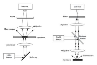
Figure 6. Optical path differences between (left) TFM and (right) EPI [24].
