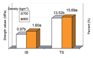
Figure 5. Effects of board density on internal bond and thickness swelling.
