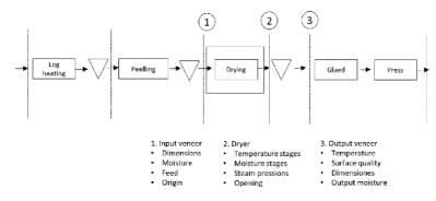
Figure 5. Data collection in a drying veneer process.
