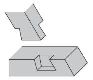
**Figure 3.** Dovetail joint (drawn by Emre ILGIN).
