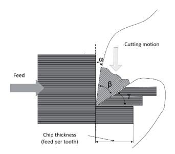
Figure 3. A typical sawmill tool and material interaction.
