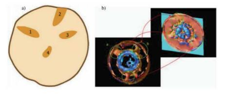
**Figure 18.** *Microwave technique used to detect knots in radial (a) and reconstructed image (b) [49].*
