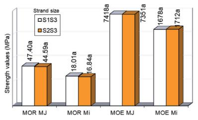
Figure 6. Effects of Strand size on bending properties.
