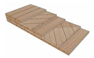
**Figure 8.** CLT panel layup with ±45° alternating transverse layer configuration (adapted from Buck et al. [10]).
