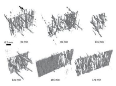
**Figure 22.** *Flow of BrPF into wood structure over time* [58].
