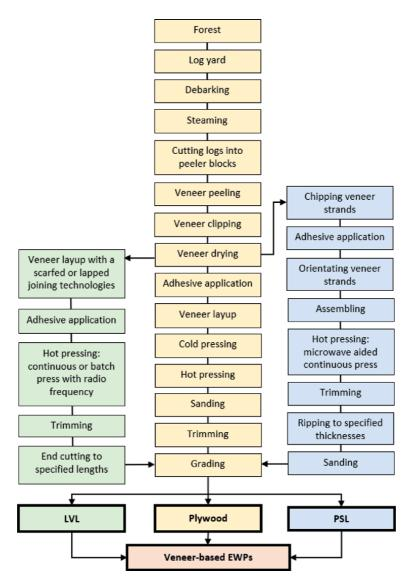
**Figure 4.** *Processes of manufacturing veneer-based EWPs.*
