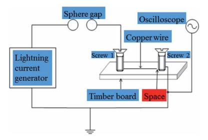
Figure 3. The schematic diagram for the experiment of the lightning strike timber.
