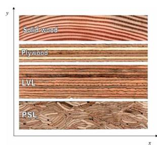
Figure 2. Cross-sections of solid wood and veneer-based EWPs.
