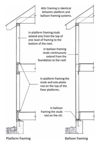
Figure 18. Light frame construction methods: platform framing and balloon framing (modified from [25]).
