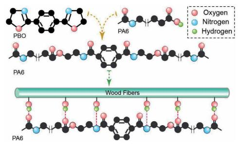
Figure 13. Reaction mechanism diagram of the chain growth of PA6 [34].
