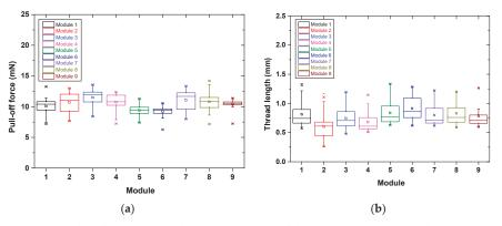
Figure 7. Comparison of 9 different modules for grease F. (a) Pull-off force and (b) thread length for 0.1 mm/s retraction speed at 30 °C.
