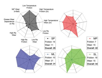
**Figure 8.** Grease ranking system based on a 1 to 4 scale (or 1 to 8 for high temperature parameters). A ranking of 4 (8) corresponds to best and 1 to worst. Low temperature is 40 °C, high temperature is 100–150 °C, low Ra is from 10–60 nm Ra, and high Ra from 120–200 nm Ra.
