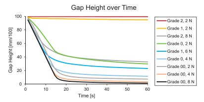
Figure 4. Rheometer gap height as a function of time for various greases and forces.
