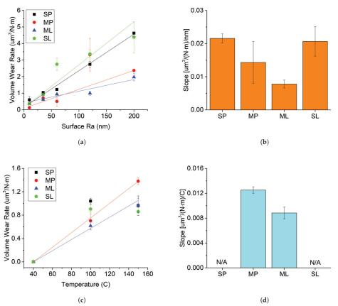
Figure 2. Wear results from EM grease ball-on-disk tests. (a) Wear rate as a function of roughness and (b) change in wear rate with roughness at 100  $^{\circ}$ C. (c) Wear rate as a function of temperature and (d) the change in wear rate with temperature at 35 nm Ra (composite Ra of 40 nm) for MP and ML.
