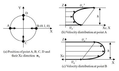
Figure 8. Explanation of the figure eight phenomenon.
