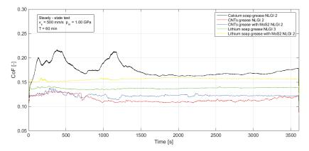
Figure 3. Friction coefficient in mixed regime under 1.00 GPa average contact pressure.
