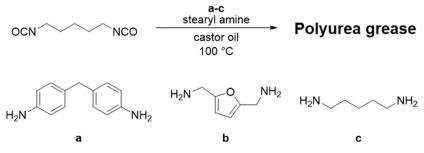
Scheme 1. Reaction scheme of polyurea grease production with all components.
