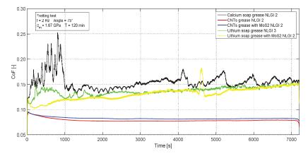
Figure 6. Friction coefficient in the fretting test under 1.67 GPa average contact pressure.
