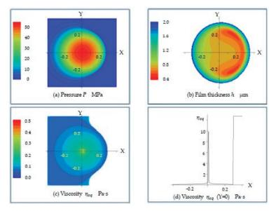
**Figure 5.** Distribution of *P*, *h*, and  $\eta_{eq}$  of grease A at a rolling velocity of 1200 mm/s.
