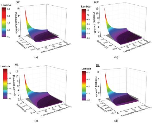
can be used as part of the design process to guide selection of a grease, surface roughness specifications, or prescribed limits on operating conditions.
