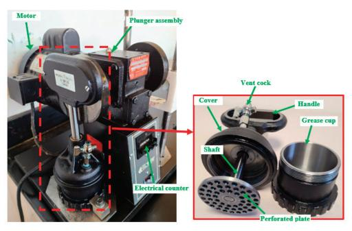
Figure 1. Modified grease worker.
