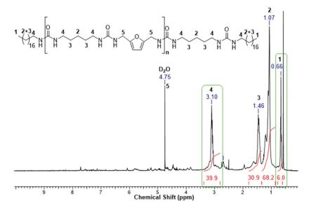
Figure 2. <sup>1</sup>H-NMR spectrum of the PDI-BAMF thickener (bio-based grease 1).
