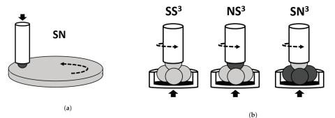
Figure 1. Greases were characterized using two test configurations: (a) Ball-on-disk and (b) 4-ball. The tests were performed with various combinations of steel (S) and silicon nitride ceramic (N) samples.
