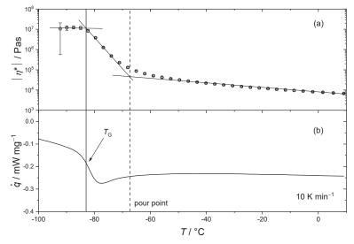
oils such as PAO8, the maximum temperature of crystal growth rate is below the glass temperature  $T_{\rm G}$  [10,11].
