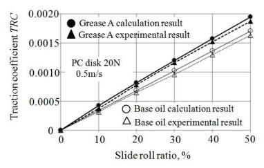
Figure 6. Comparison of the traction coefficient between the calculation and the experiment.
