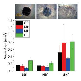
Figure 4. Wear area for four greases and three bearing configurations measured using the 4-ball test. Representative wear patterns (from left to right):  $SS^3$  circular wear scar on steel ball,  $NS^3$  circular wear scar on steel ball, and  $SN^3$  elliptical wear scar on ceramic ball.
