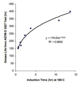
Figure 1. Induction time vs. grease life (ASTM D 3527 Test) [14].
