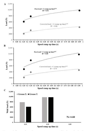
**Figure 3.** Influence of speed ramp up time on corrected load, pass load and weld load for grease X and Y. A correlation between speed ramp up time and load (corrected load and pass load) for grease X (**A**) and grease Y (**B**), and the changes in weld load due to ramp up time for grease X and Y (**C**). All the measurements were in duplicate.
