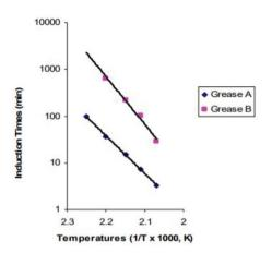
Figure 2. Temperature effects on induction time [14].
