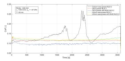
Figure 5. Friction coefficient in mixed regime under 1.67 GPa average contact pressure.
