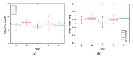
Figure 8. Comparison of (a) pull-off force and (b) thread length between 5 different users for the same modules for grease G. Test conditions: 0.1 mm/s retraction speed at 30 °C.
