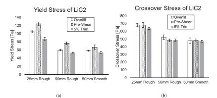
**Figure 6.** Comparison of (**a**) yield stress and (**b**) crossover stress of LiC2 worked for 60 strokes using an overfilled sample compared to a pre-sheared sample compared to a standard 5% trim.
