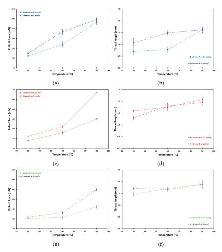
Figure 4. Effect of temperature and retraction on the pull-off force and thread formation of greases (a,b) A, (c,d) B and (e,f) C.
