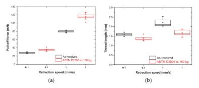
Figure 9. Effect of 4-ball wear testing (ASTM D2596) on the (a) pull-off force (adhesion) and (b) thread length (tackiness) of grease H.
