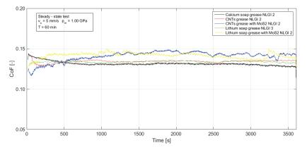
Figure 2. Friction coefficient in boundary regime under 1.00 GPa average contact pressure.
