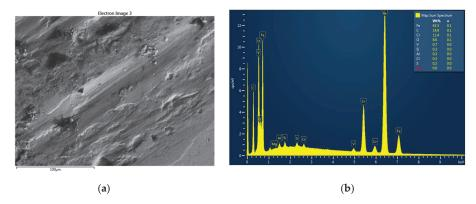
Figure 7. (a) SEM image of a worn surface ball of steel ball: Calcium soap grease; (b) EDX spectrum: Calcium soap grease.
