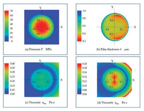
pure rolling case, where  $\Delta U$  is 0, Equation (57) results in Equation (58). It can be understood that in such a case, no figure-eight-shaped distribution appears as is shown in Figure 5c.
