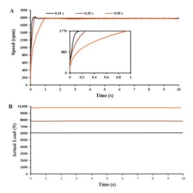
**Figure 2.** Measurement and controls for speed ramp up time and normal load in a Ducom four-ball tester. Real time changes in the speed profiles (**A**) and load profiles (**B**) at ramp up time of 0.15 s, 0.25 s and 0.95 s. Note: Ramp up time is the time taken to reach the average speed of 1770 rpm (average speed follows ASTM D2596-15, see the figure inset) and the motor was designed for full torque or load at zero speed.
