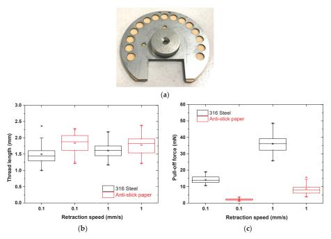
**Figure 5.** (a) Grease scoop with anti-stick paper. Effect of anti-stick paper on the (b) thread formation (tackiness) and (c) pull-off force (adhesion) of grease D for 0.1 and 1 mm/s retraction speed at 30 °C.
