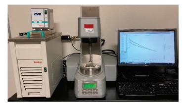
Figure 2. Anton Paar MCR 301 rheometer used in experiments
