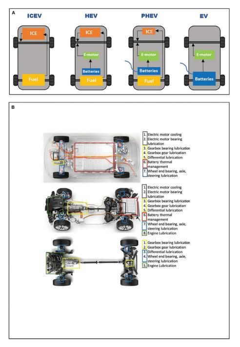
Figure 3. (A) Comparison of battery and ICE sizes and (B) an image of the main areas where lubrication is required in an EV (Tesla), hybrid electric vehicle (HEV) (Volkswagen NetCarShow), and ICEV (Subaru Forester showroom), respectively [15].
