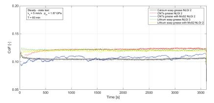
Figure 4. Friction coefficient in boundary regime under 1.67 GPa average contact pressure.
