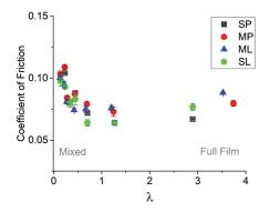
Figure 5. Stribeck curve based on measured friction and calculated  $\lambda$  ratios for four greases tested across all roughness and temperature conditions.
