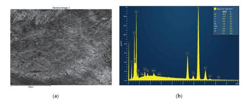
Figure 8. (a) SEM image of a worn surface ball of steel ball: CNTs based grease with MoS<sub>2</sub>; (b) EDX spectrum: CNTs based grease with MoS<sub>2</sub>.
