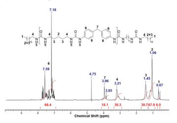
Figure A2. <sup>1</sup>H-NMR spectrum of the PDI-MDA thickener.
