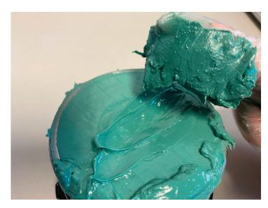
Figure 13. Smooth texture of worked grease in the cup below compared to the rough texture of unworked grease above it.
