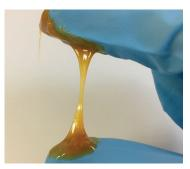
Figure 1. Thread formation during physical separation of a grease.
