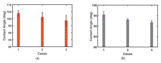
Figure 8. Contact angle for Li-P and CaS greases for different cases: (a) Li-P; (b) CaS.
