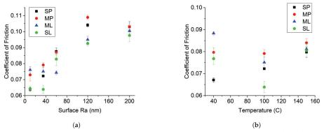
**Figure 3.** Friction results from EM grease ball-on-disk tests. Friction coefficient (**a**) as a function of surface roughness at 100  $^{\circ}$ C and (**b**) as a function of temperature at 35 nm Ra (composite Ra of 40 nm).
