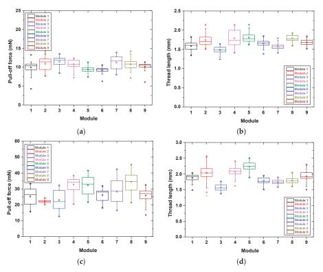
Figure 6. Comparison of 9 different modules for grease E. (a) Pull-off force and (b) thread length for 0.1 mm/s retraction speed at 30 °C. (c) Pull-off force and (d) thread length for 1 mm/s retraction speed at 30 °C.
