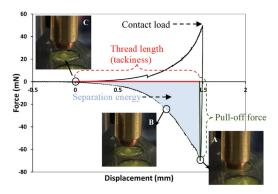
Figure 2. An indicative indentation-retraction curve and measured values.
