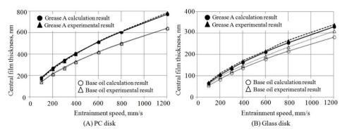
Figure 4. Comparison of film thickness between the calculation and the experiment.
