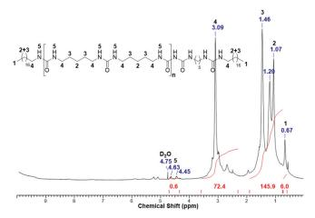
Figure A1. <sup>1</sup>H-NMR spectrum of the PDI-PDA thickener.
