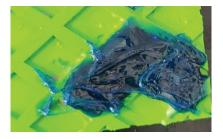
Step 3: Remove the excess grease. The grease is reapplied if air bubbles are entrapped in the grease.
