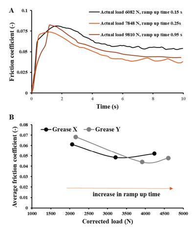
**Figure 4.** Influence of speed ramp up time on friction for grease X and Y. Real time changes in the friction profiles for grease X (**A**) and the relationship between average friction coefficient and corrected load due to an increase in ramp up time (**B**). All the measurements were in duplicate.
