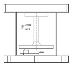
Figure 1. Ball on disk setup and rotational tribometer.
