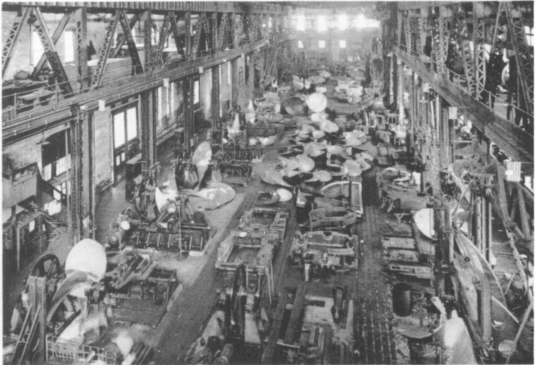
Cramp's Propeller Foundry in World War I. This photograph shows destroyer propellers undergoing finishing process in the main bay. Cramp's Shipyard War Activities (Philadelphia, 1919). Historical Society of Pennsylvania
