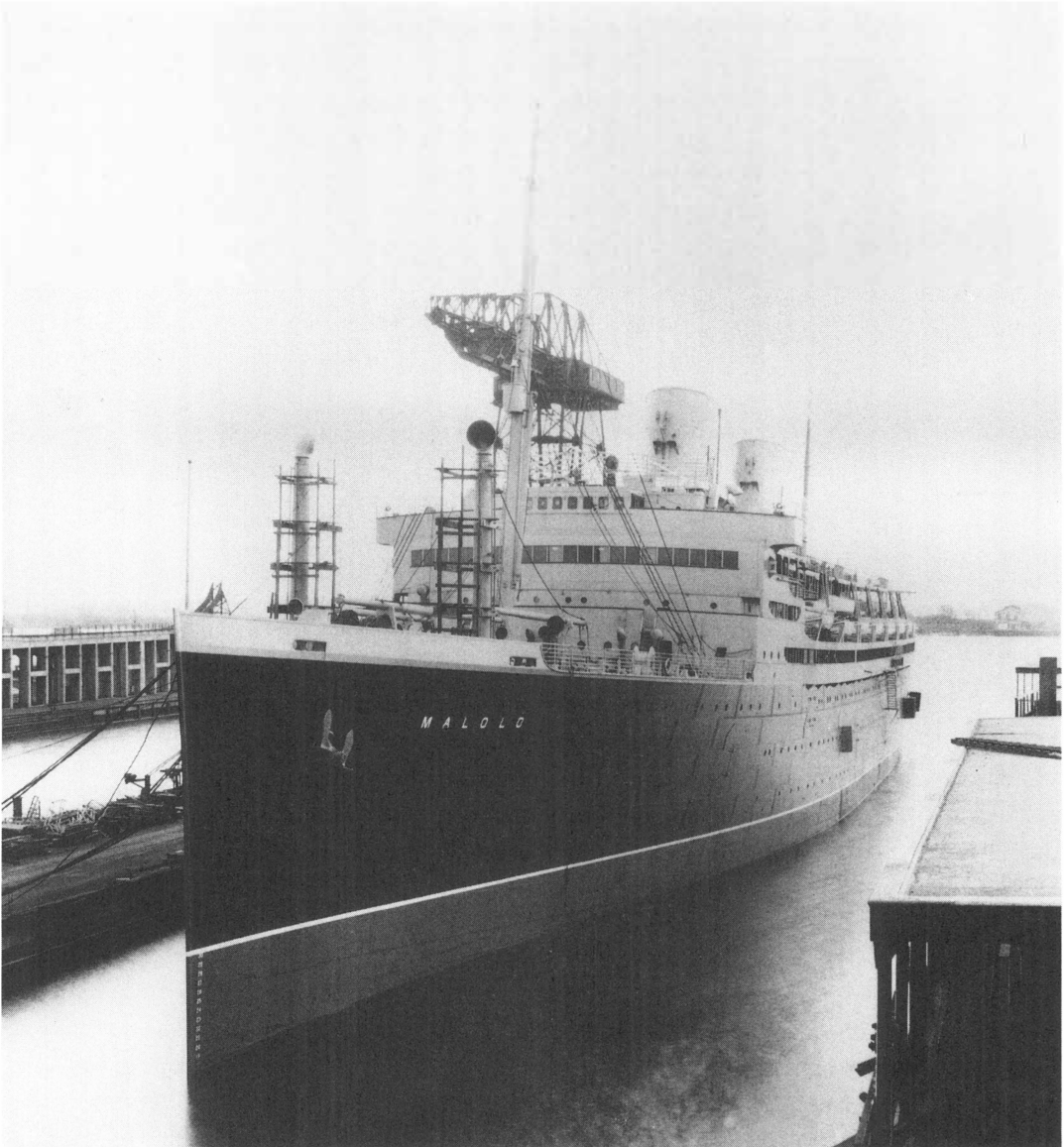
Passenger liner Malolo outfitting at Cramp, April 5, 1927. The largest and most luxurious American passenger liner of her time, the Malolo boasted two movie theaters, a swimming pool, and a gymnasium. The De La Vergne Machine Company, Cramp's new subsidiary, supplied turbine reduction gear for each of her two 12,500-horsepower turbines, which ran at 1,500 rpm and had to be geared down to turn the propeller at 125 rpm. To compensate for the lack of alcoholic beverages aboard this Prohibition-era vessel, the builders installed a custom-made soda fountain, where a "bartender" could mix any soft drink imaginable. Franklin Institute Cramp Shipbuilding Co. Collection, Independence Seaport Museums through the Pew Museum Loan Program
