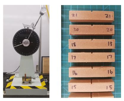
Figure 5. Impact Testing Setup (Left) and Examples of Impact Testing Specimens (Right).
