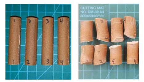
Figure 4. Example Compression Specimens Before (Left) and After (Right) Testing.
