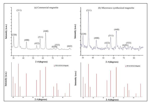
**Figure 1.** X-ray diffraction spectra of (**a**) commercially available magnetite particles and (**b**) the microwave-synthesized magnetite particles.
