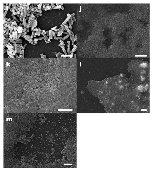
**Figure 3.** SEM of the nanomagnetite particles obtained in experiments: (a) 1; (b) 2; (c) 3; (d) 4; (e) 5; (f) 6; (g) 7; (h) 8; (i) 9; (j) 10; (k) 11; (l) 13; (m) 12 and 14. White bar length = 1  $\mu$ m.
