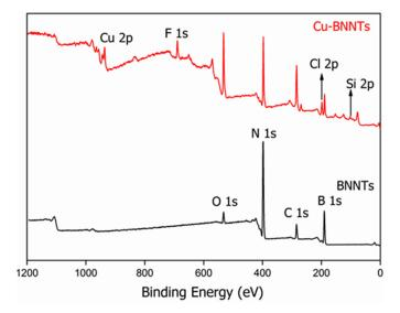
Figure 4. Survey XPS spectra for BNNTs and Cu-BNNTs.
