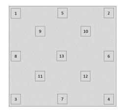
**Figure A2.** Imaging convention for each coupon in the experiment. Regions were chosen to reflect the corners (1–4), edges (5–8), central area (9–12), and absolute center (13) of each sample.
