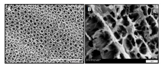
Figure 1. Aligned titanium nanotubes (TiNT) (A) and trabecular TiNT (B) surfaces. (A,B) Scale Bar: 1 µm.
