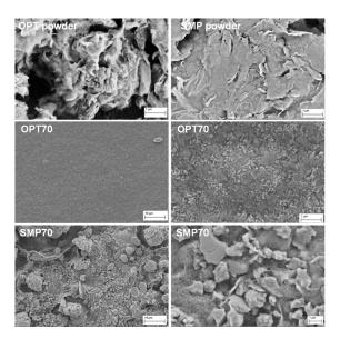
**Figure 1.** SEM micrographs of the food-grade activated montmorillonite (Optigel, OPT) and high-purity unmodified montmorillonite (SMP) powders, and the OPT- and SMP-based films.
