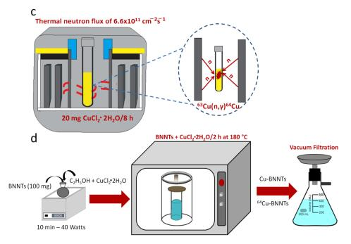
**Figure 1.** Schematic representation of synthesis of the BNNTS (**a**), purification process (**b**), activation process of  $CuCl_2 \cdot 2H_2O$  to obtainment of <sup>64</sup>Cu radioisotope (**c**) and incorporation of Cu and <sup>64</sup>Cu into BNNTs samples (**d**).
