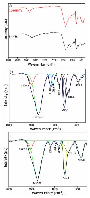
Figure 2. Infrared spectra of (a) BNNTs and Cu-BNNTs in the region between 4500 and 60 cm<sup>-1</sup>.
