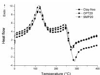
Figure 2. Differential scanning calorimetry (DSC) thermograms of Clay-free, OPT20 and SMP20 samples.
