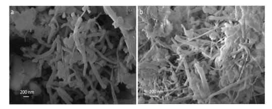
Figure 7. SEM images of BNNTs (a) and Cu-BNNTs (b).
