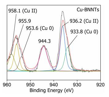
Figure 6. High-resolution spectrum XPS for Cu-BNNTs.
