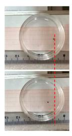
Figure 4. Ferrofluid microdroplet being pushed in oleic acid.
