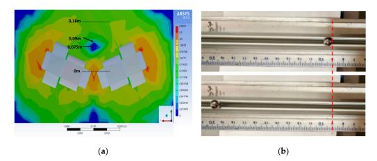
**Figure 3.** (a) Map of magnetic forces generated around the electromagnets; units reported in the simulation are arbitrary and are intended to highlight areas where the force is almost zero (dark blue), while the other colors indicate forces >0. The scale bar is in meters. (b) A paramagnetic sphere pushed from 9 to 19 cm on an aluminum rail using the actuator system.
