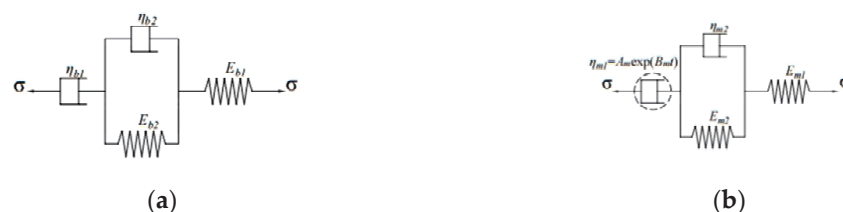
Figure 3. Creep compliance fitting model: (a) the Burgers model; (b) the modified Burgers model.
