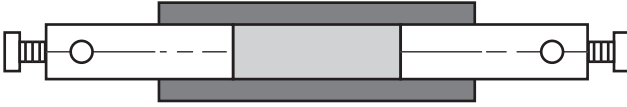
Fig. 6. Branley Coherer, 1902. Inside an evacuated glass tube are metal filings. Silver plugs act as terminals and enclose the filings by capping the open ends of the glass tube. Detail from figure in Ray Stannard Baker, “Marconi’s Achievement: Telegraphing across the Ocean without Wires,” McClure’s Magazine , February 1902, 291.
