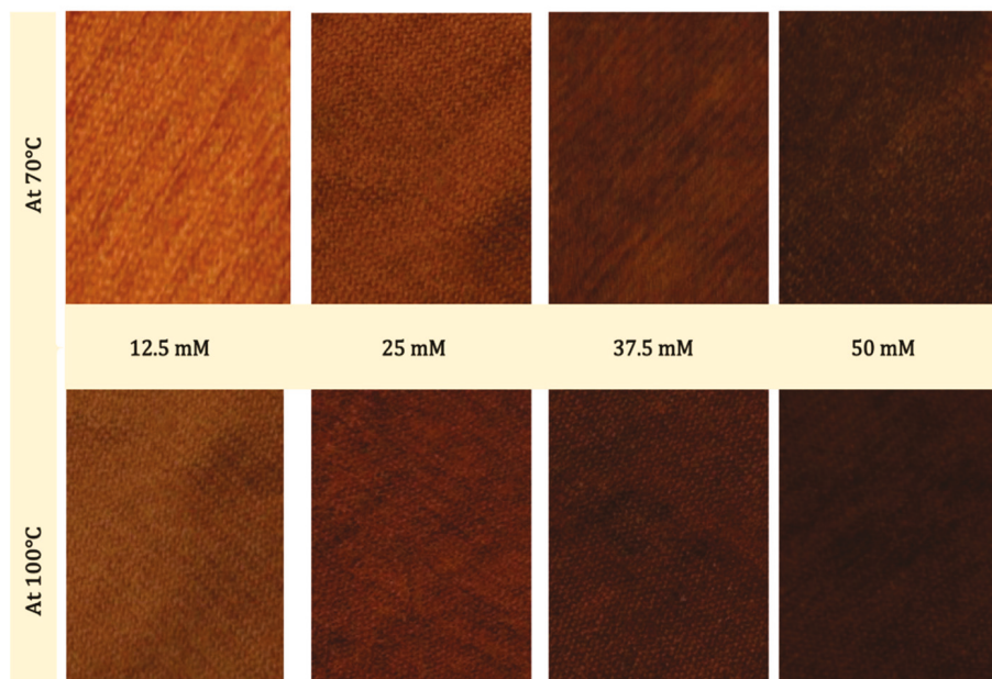
Figure 6. Photographs of Se-dyed wool fabrics with different concentrations of synthesized Se-NPs at 70 °C and 100 °C.
