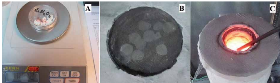
Figure 5. Preparation of ZnAl_2O_4 catalysts: A – Weighting; B – Insertion in the metal matrix; C – Initial testing with and without catalysts.
