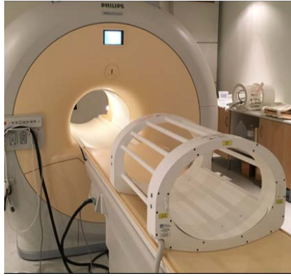
Figure 2.6: ^{19}\text{F}/^1\text{H} elliptical birdcage coil (Rapid Biomedical, Rimpar, Germany) used in the LIFT study, shown in situ on the MRI scanner bed at the NMRC, Newcastle University.
