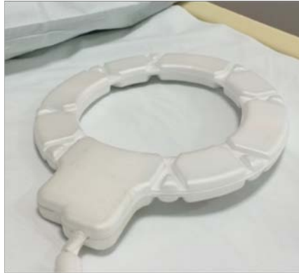
Figure 2.8: ^{19}\text{F} surface coil (PulseTeq Ltd., Woking, UK) used in the LungGas study.
