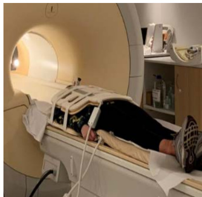
Figure 2.7: 8-element ^1\text{H} receive array coil (Philips Healthcare, Best, The Netherlands) used in the VQ MRI study, shown with a study participant in situ .
