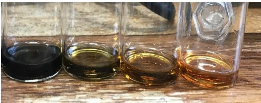
Figure 4.27: Photograph of collected post reaction samples at 150, 130, 110 and 90 °C (from left to right).
