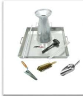
*Fuente: Material test equipments Slump Cone Test Set*
