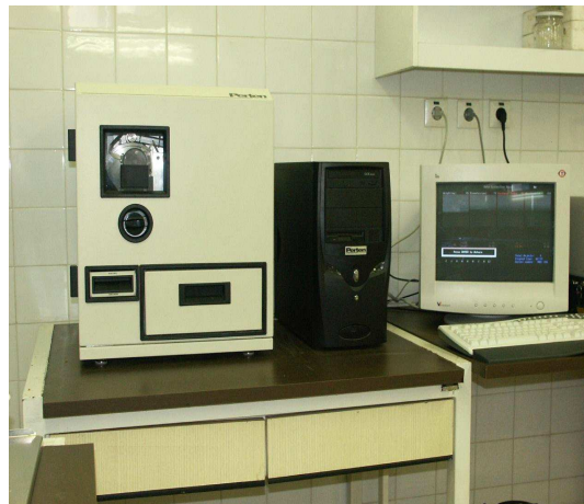
Figure 1. SKCS 4100 instrument (Perten, Inc.)
