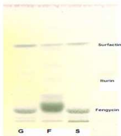
Figure 2. Influence of some carbon source on the antibiotic production of B. subtilis B23 analysed by TLC. G= glucose, F= fructose, S= saccharose. The nitrogen source was glutamic acid.
