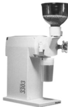
Figure 2. Perten 3303 disc mill (Perten, Inc.)
