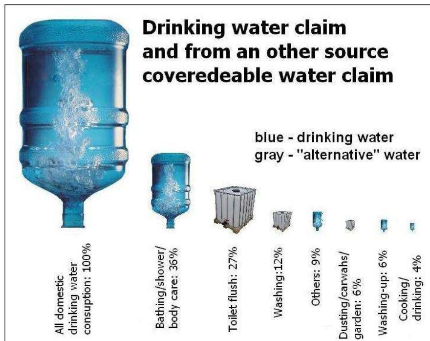
Fig. 1. Structure of household drinking water consumption, replaceable and non replaceable water demand (own picture, based on BDEW data)
