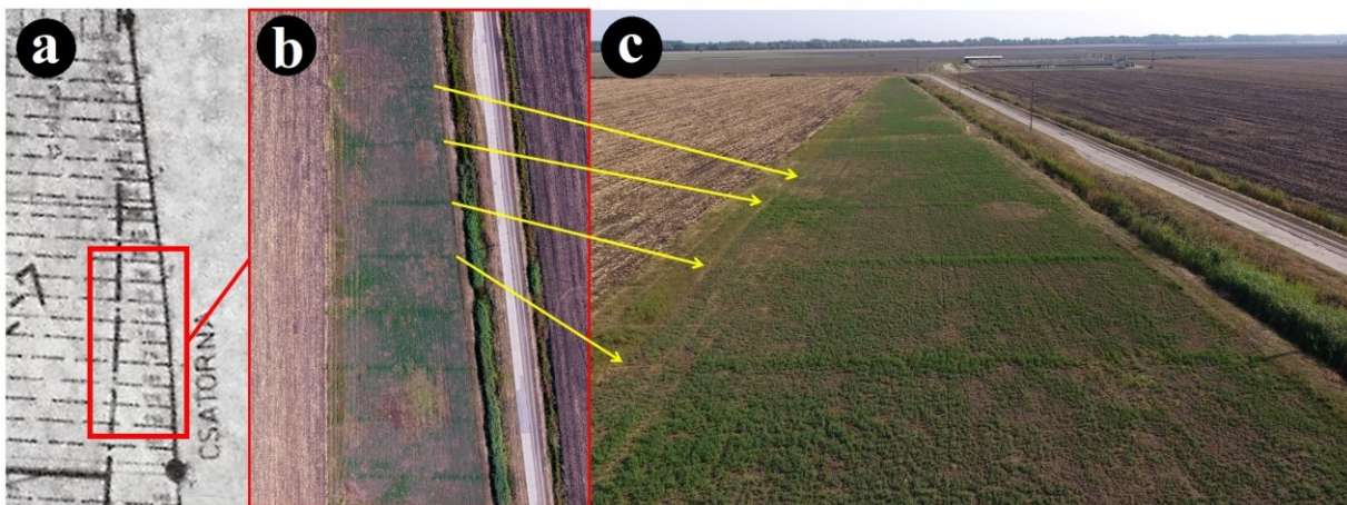
Fig. 6 Phenological differences in alfalfa plants over drains and the intermediate areas: (a) blueprint of the tile drains, (b) vertical aerial photo of the alfalfa field (UAV), (c) oblique aerial photo of the alfalfa field, where denser vegetation indicates the lines of the drain (UAV)
