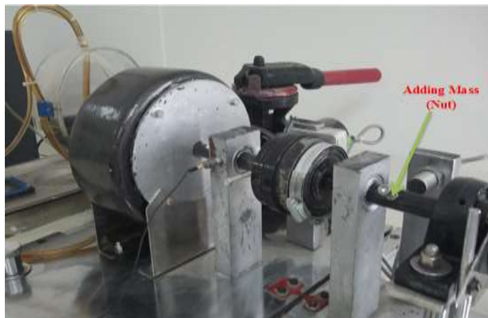
Figure 6. Adding extra mass to simulating unbalance.
