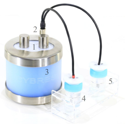
Fig. 1. The differential EIS spectrometer, 1,2,3 – elements of the device; 4, 5 – electrodes of the channel 1 and 2.
