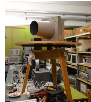
Fig. 1: The rotation speaker from Stockhausen's KONTAKTE at the WDR Studio for Electronic Music in Cologne, DE
