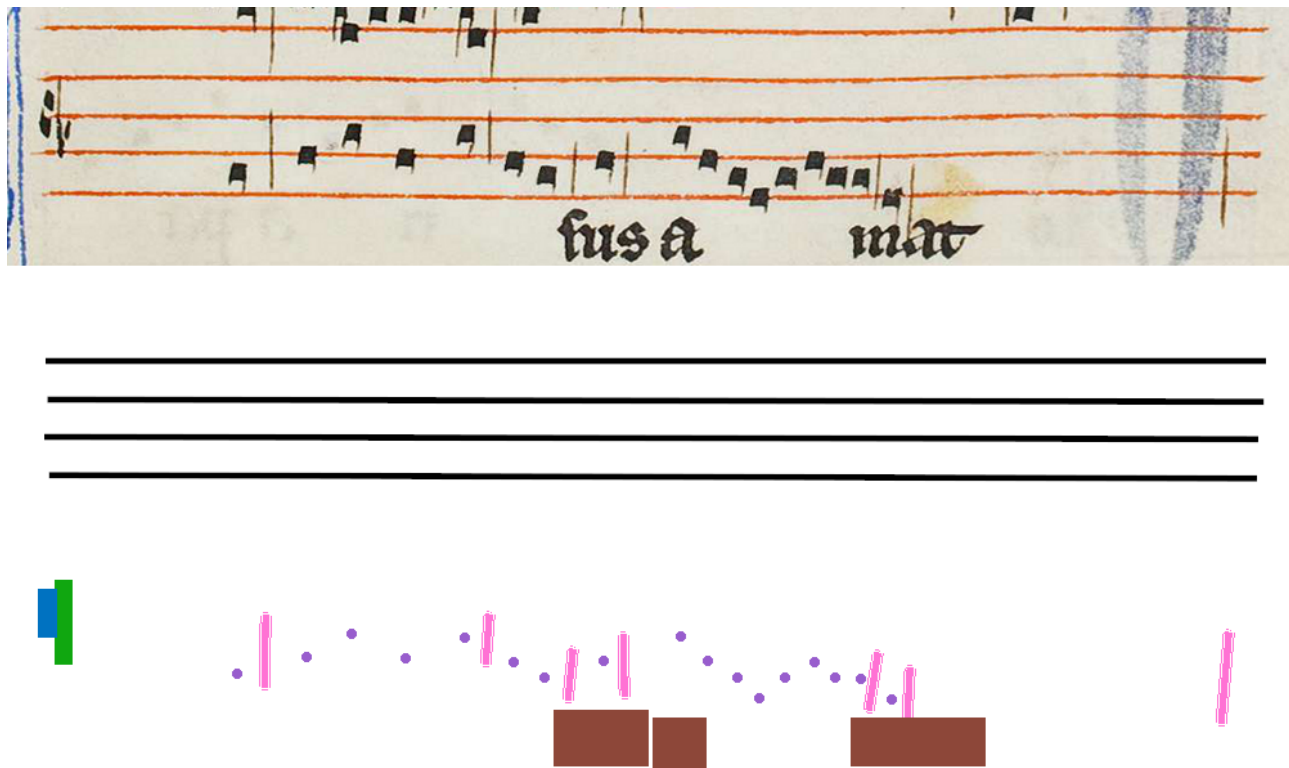
Figure 4: Transformed staff (top), ground truth staff lines mask (middle) and item mask (bottom). The sizes of the mask items are balanced as hyperparameters.
