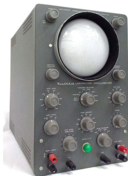
Figure 1: Heathkit oscilloscope model O-12 with 5-inch tube, ca. 1958. Photo by the author. Licensed under CC BY-NC-SA 4.0.
