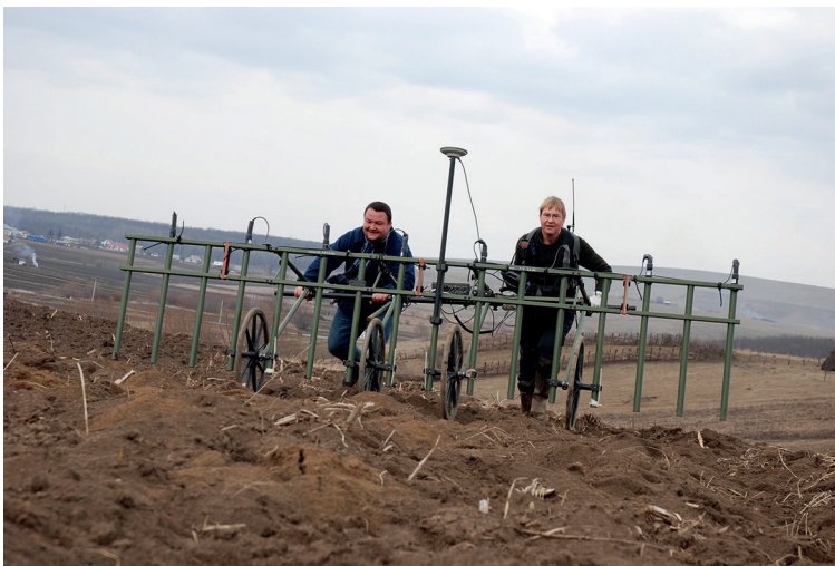
Fig. 9 The geomagnetic device of the Kiel Graduate School “Human Development in Landscapes” during its use in Baia.
