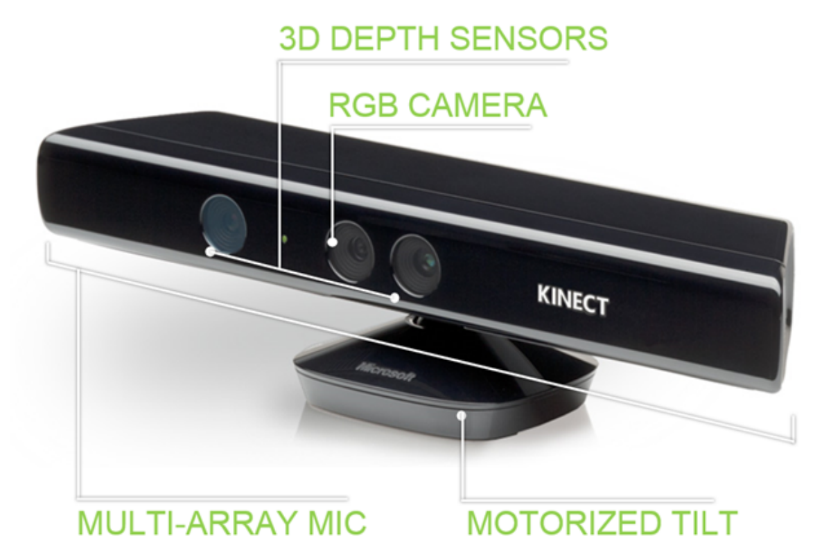
Figure 1: Microsoft Kinect hardware features—version 1.7 of the device. Available from http://blogs.msdn.com/b/msgulfcommunity/archive/2013/06/05/kinect-for-windows-sdk-part-i.aspx , June 5, 2013.
