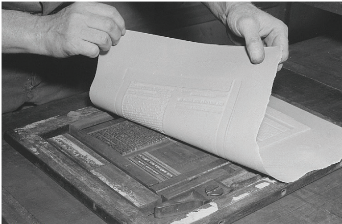
A flong is made from a forme of type; the stereotype printing plate will then be cast from the flong Photograph courtesy of Deutsche Fotothek
