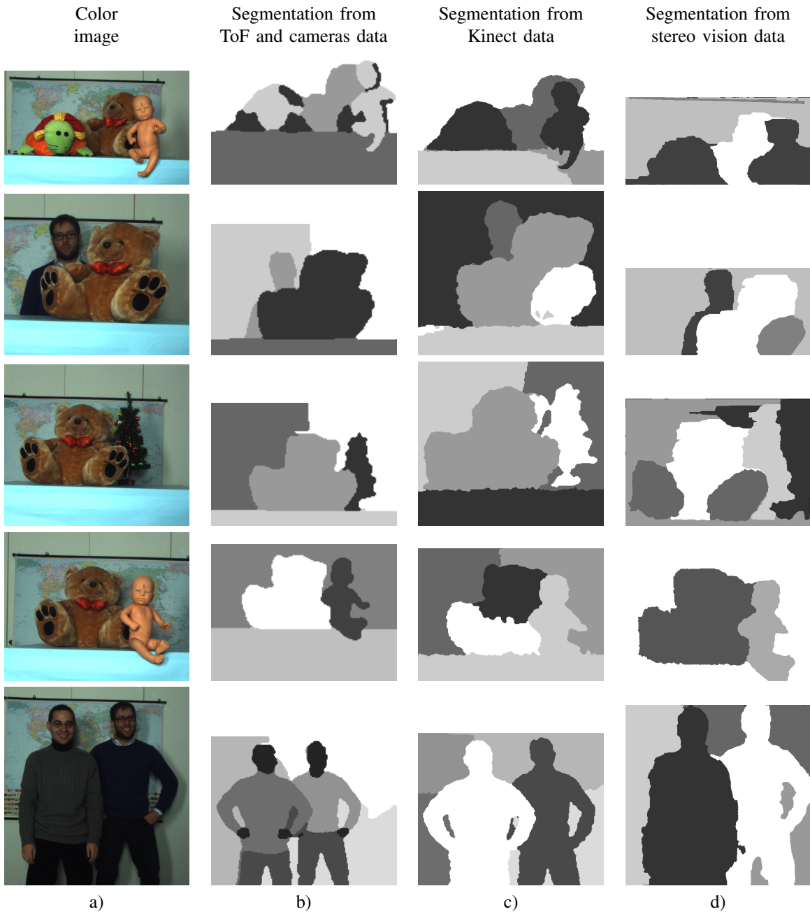
Fig. 18. Segmentation of some samples scenes exploiting depth data coming from different acquisition systems: a) color image of the scene; b) segmentation from the ToF camera data and the color images provided by the trinocular setup; c) segmentation from the Kinect data; d) Segmentation from the stereo vision data.
